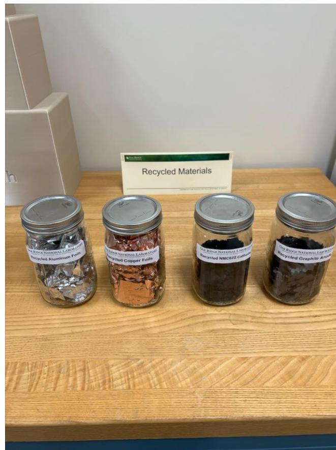
Recycled Materials: Aluminum Foils, Copper Foils, NMC622 Cathode, Graphite (Anode)
