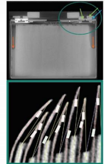
EV battery appears fine, but further inspection shows electrode bending
