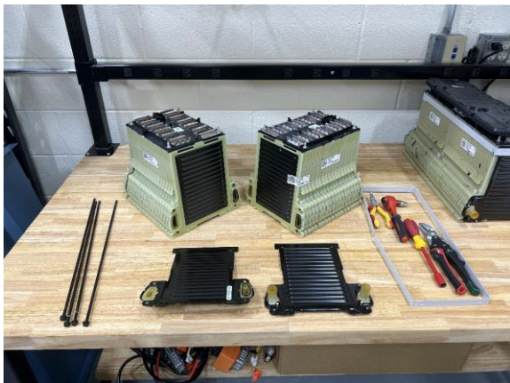
Chevy Volt Modules and structural components
