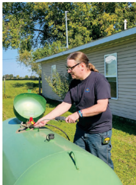
Left: Jeremy Truog, Technical Manager and Building Performance Institute (BPI) Certified Energy Auditor performs a blower door test on a home during an energy audit. A blower door is a machine that tests the air tightness of a home and helps measure how much air is entering or escaping from it. Center: Jeremy checks a propane tank for gas leaks during an energy audit. Right: Jeremy runs diagnostics on a home’s furnace during an energy audit. Photo: Northwest Michigan Community Action Agency
