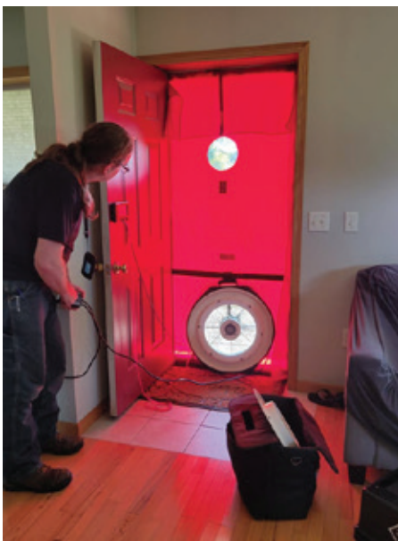
Left: Jeremy Truog, Technical Manager and Building Performance Institute (BPI) Certified Energy Auditor performs a blower door test on a home during an energy audit. A blower door is a machine that tests the air tightness of a home and helps measure how much air is entering or escaping from it. Center: Jeremy checks a propane tank for gas leaks during an energy audit. Right: Jeremy runs diagnostics on a home’s furnace during an energy audit. Photo: Northwest Michigan Community Action Agency
