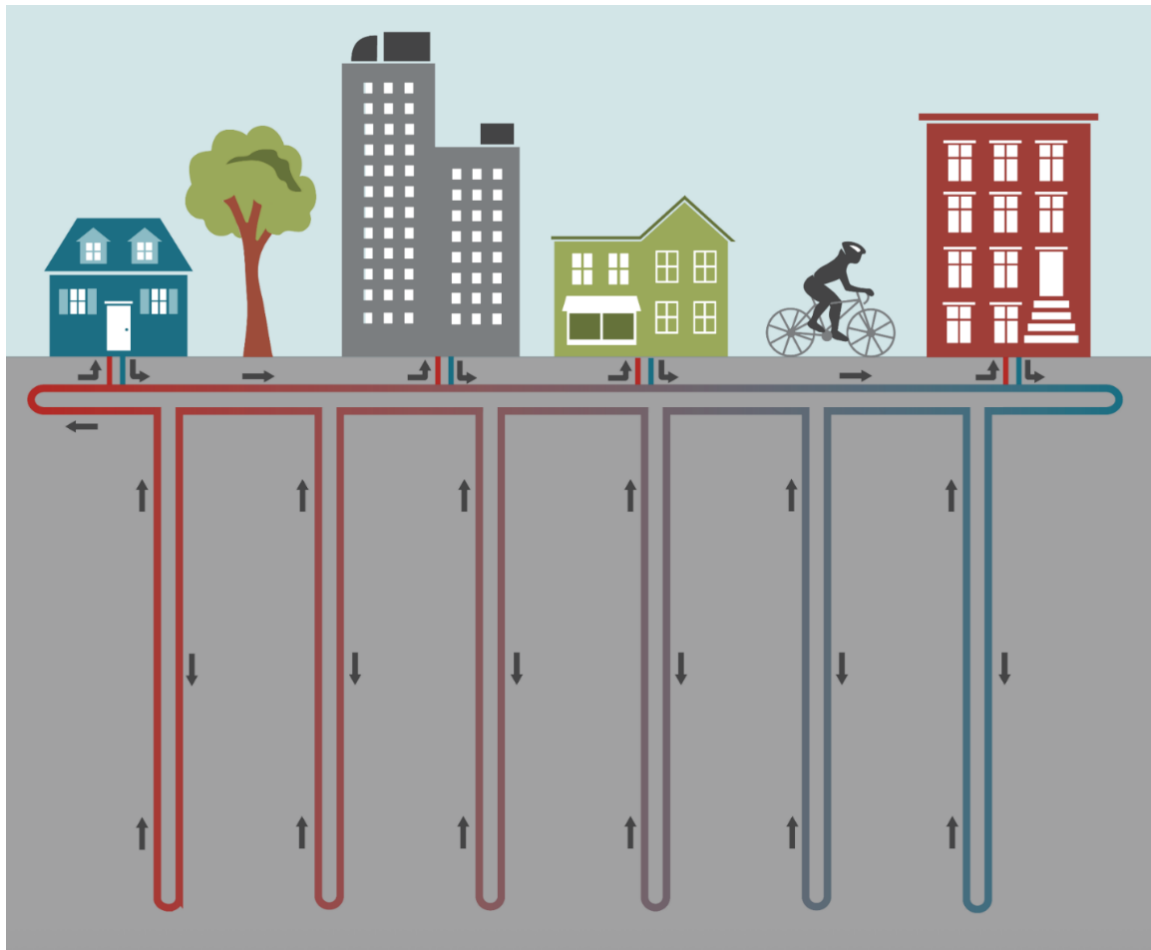
Figure 1. Example of a networked geothermal system.
