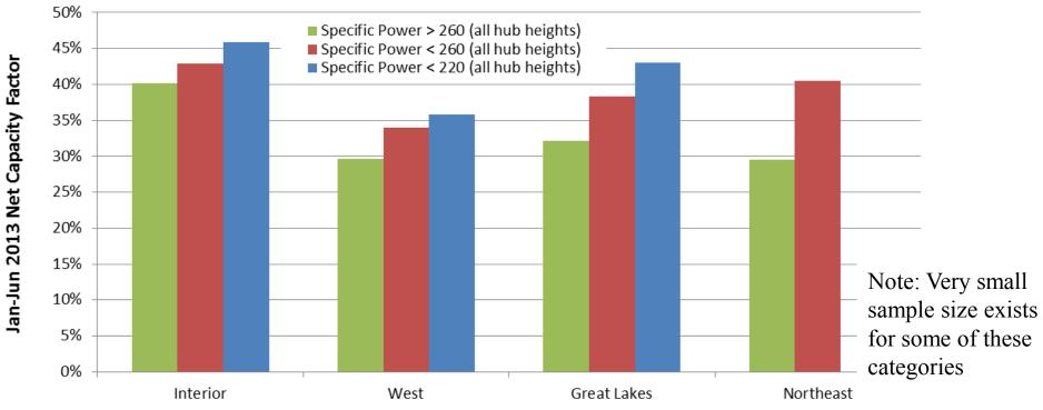
Specific Power < 260 = recent, lower wind-speed models such as GE 1.6 MW / 100m rotor; Siemens 2.3/108; Vestas 1.8/100; Nordex 2.4/117; Specific Power < 220 = GE 1.6/100 24
